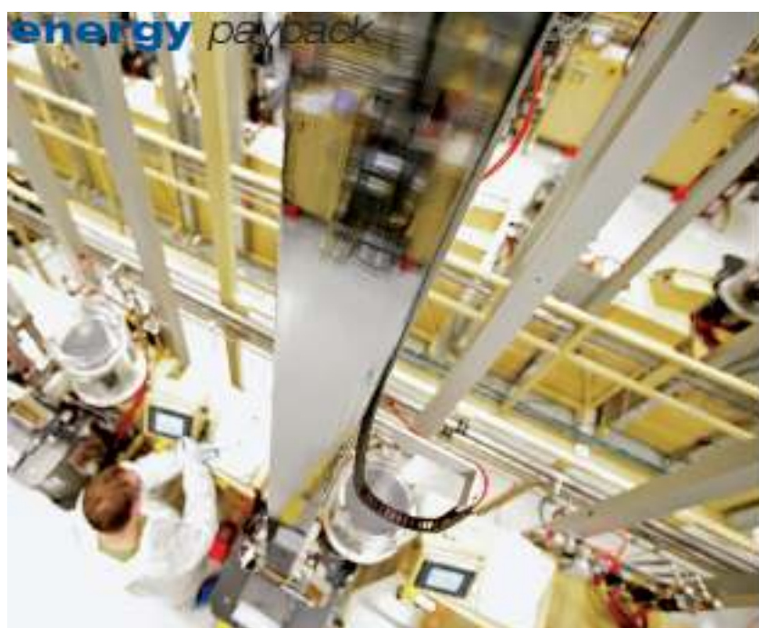
The Evergreen Solar manufacturing process grows string-ribbon crystals at the thickness of the finished cell, saving silicon waste and reducing embodied energy by as much as 25%.
